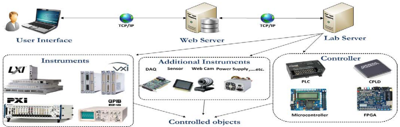
Figure 1. Common Generic Architecture design of today's remote laboratory for industrial electronics applications.
